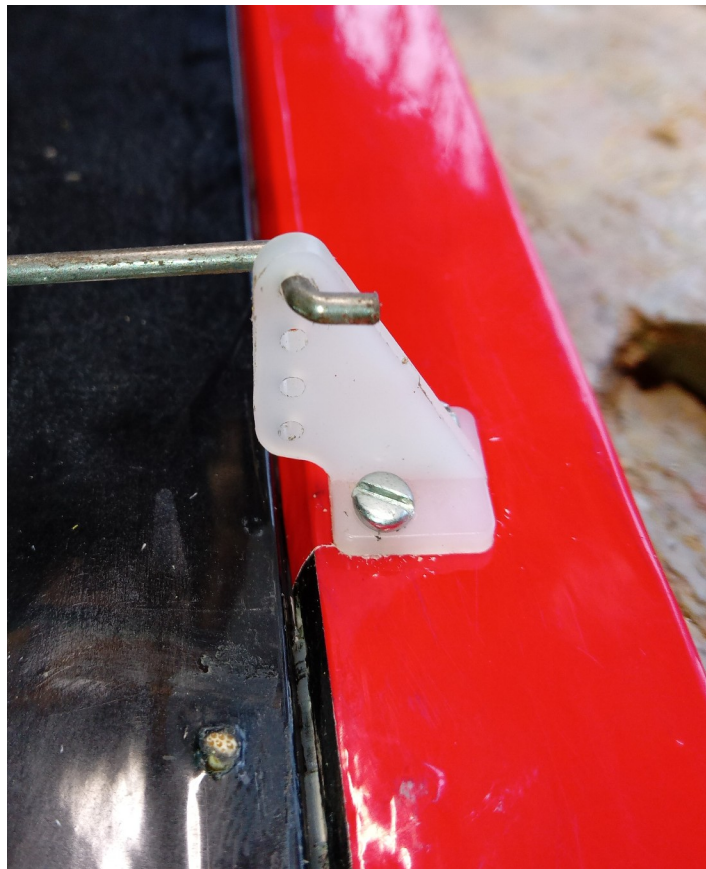
Horn Aligned With Hinge Line
