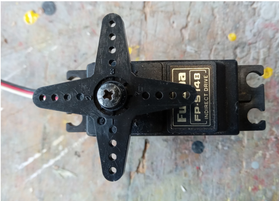
Servo Arm in correct position when Tx stick is centered
