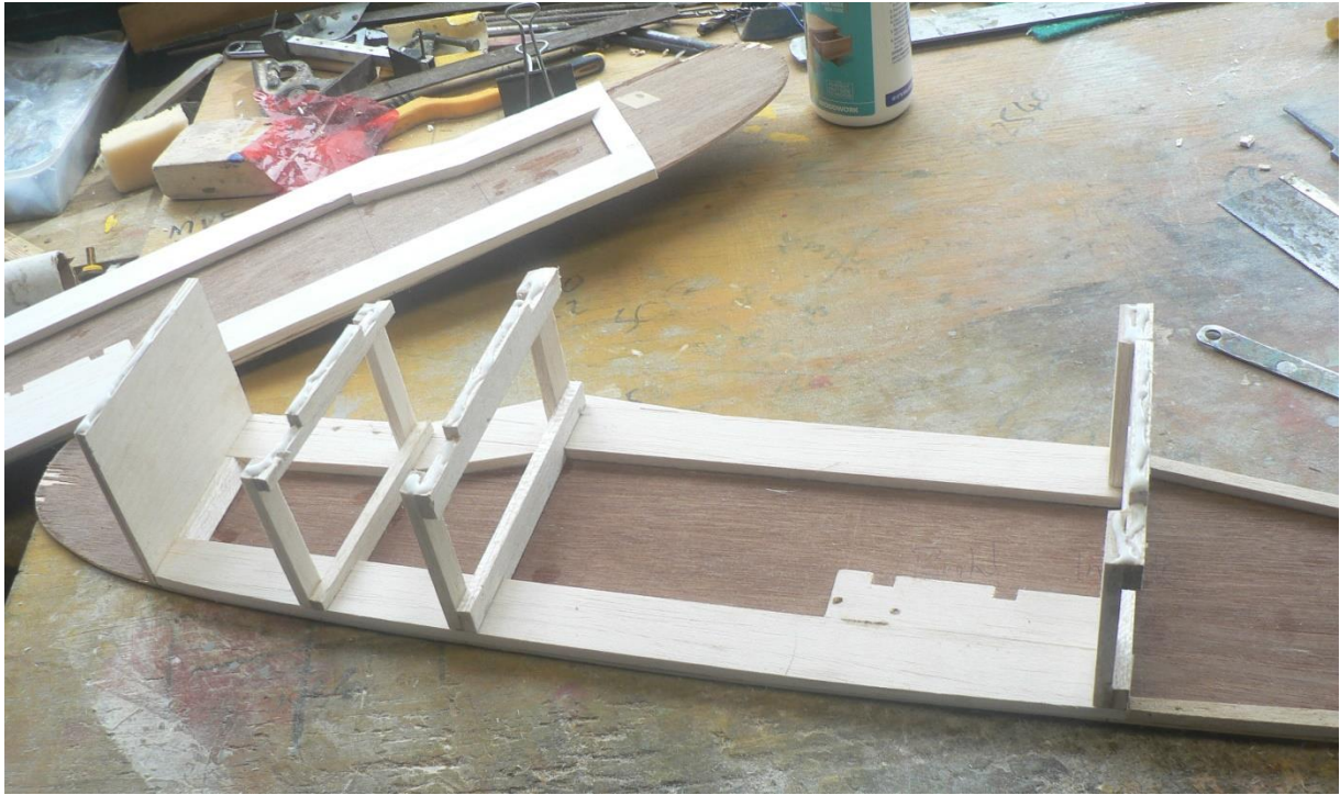
Formers and firewall set up
