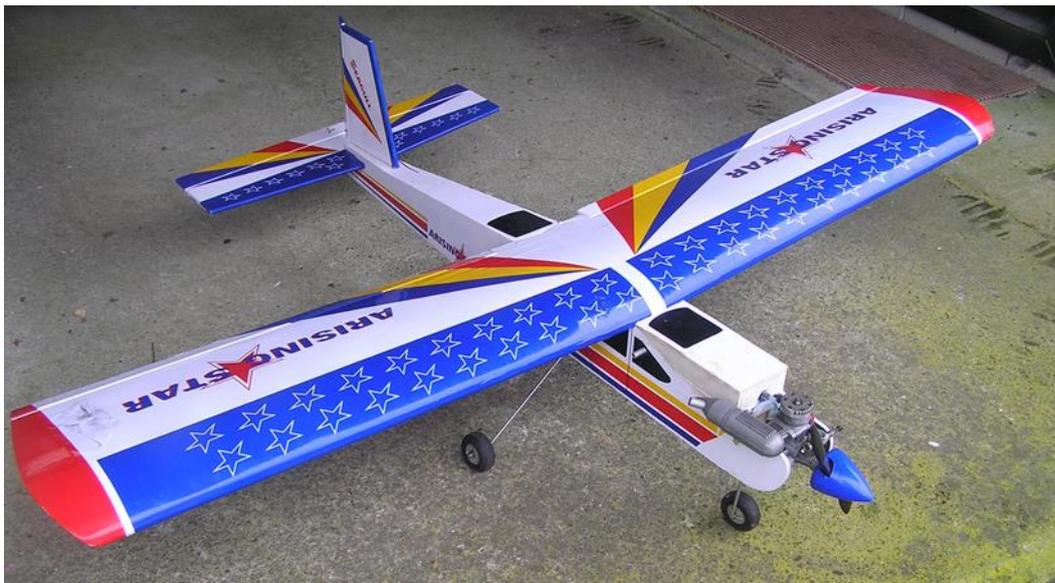
The SC 40 up front is a clone of an OS 40FSR. Unfortunately like ASP and others the carb is not made to the standards of an OS one. It was quickly reengined with an OS 40FP and is going very well. Meanwhile the SC carb has had both needles polished with 1500 emery paper and after much fiddling about in the test stand a reliable idle and transition from slow to fast has been achieved.
