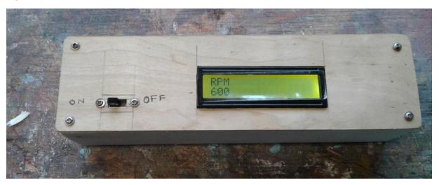
My dabbling into the world of Aduino has now produced somethig useful. A rev counter. It is based on an Arduino Naro and an LCD display. An LDR changes resistance every time a prop blade goes past and forms part of a potental diver which is AC coupled to an op amp acting as a comparator. The output of the comparator is a string of pulsed which are counted by the Arduino which is programmed to converted the pulses to rpm displayed on the LCD display
