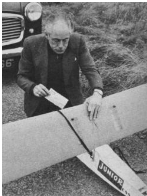
Sid Allen, noted British RC flier, placing air mail letter aboard. Note the two transparent fuel tanks in wing.
