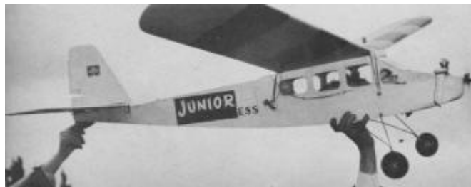
No beauty, the first across-the-channel plane is an ED kit, popular abroad. The radio is an ED Mk. 4 three-tube type, making an all ED project.
