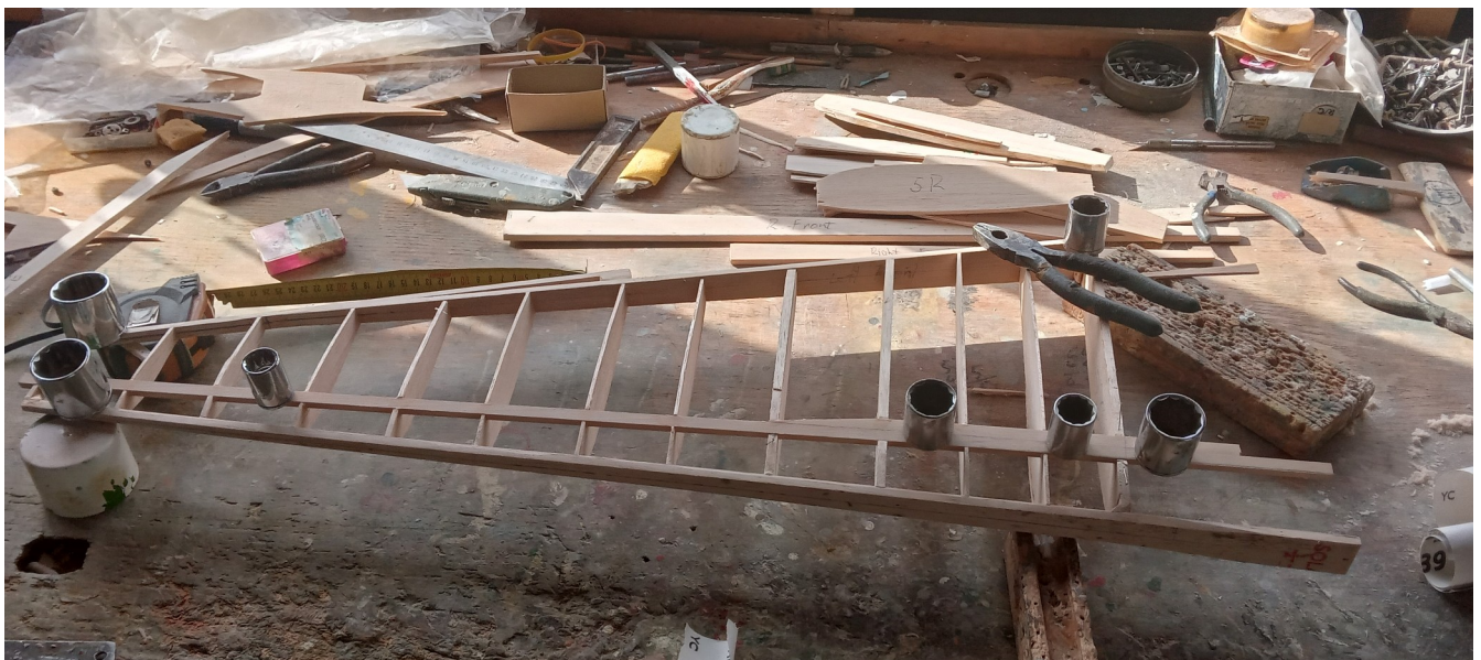
Start of wing jigged to incorporate washout
